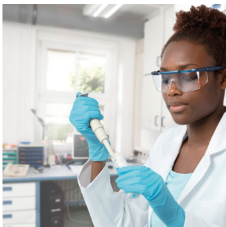
FIGURE 1.3.1 A lab coat, gloves and safety glasses are essential items of personal protective equipment in the laboratory.
