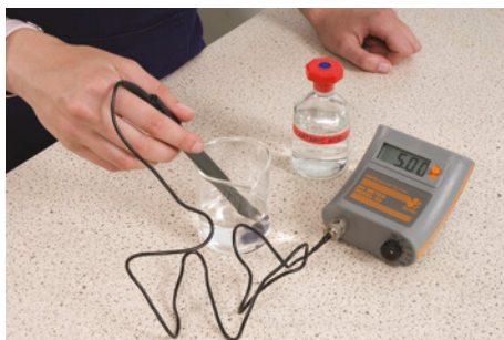
FIGURE 1.3.9 A student measures the pH level of tartaric acid using a pH meter. To ensure an accurate reading, the student would first have calibrated the meter using standard solutions of known pH.
